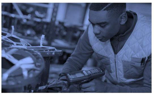
Parts/assemblies are scanned as they are received into inventory and again, when consumed – automatically sending demand signals for replenishment.
